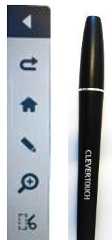
The screen is responsive to touch with a hand/finger and will register up to 20 points of contact on the screen simultaneously if you would like multiple drawers/writers to use the screen at once. There is also a special pen which can be used upon the screen. The pen is usually located on the side edge of the display.
