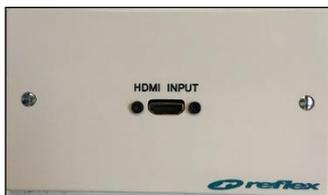
Use an appropriate cable to carefully connect your device to the HDMI socket making sure the cable is securely in at both ends. Sometimes a poor connection will result in picture but no sound, in which case try connecting the cable again.
