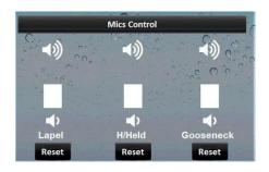
Any of the mic levels can be reset to its default level by pressing its associated Reset button.
