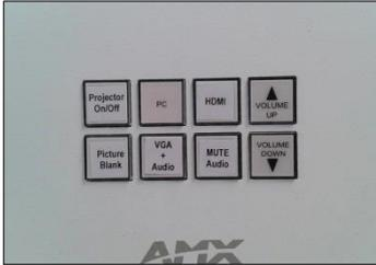
The Projector and audio is controlled from the AMX control panel on top of the lectern.
