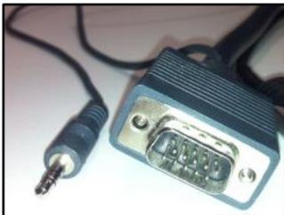
Plug your laptop into the VGA+audio cable that is available on the top of the lectern. When there is a device connected to this cable it over-rides the signal from the PC in the lectern – therefore to operate the projector and amplifier follow the same instructions as for PC above.
