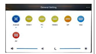
Choose a source by tapping on it. The blue dots below a source show which are currently active (i.e. available and connected). There are also volume and screen brightness controls available on the General Setting screen.
