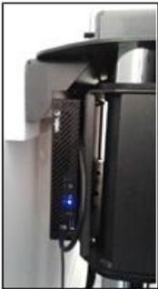
A micro PC is currently located behind the display and must be switched on manually. NB: The USB socket in the connection plate on the wall can connect USB devices connects to the PC.
