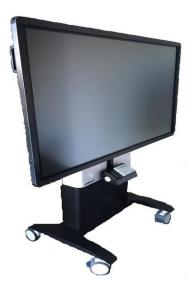
This is a large format touch screen which responds to either your hands or to pens that should be located at each edge of the screen. The screen has a Crestron controller from which most functions can be selected.
