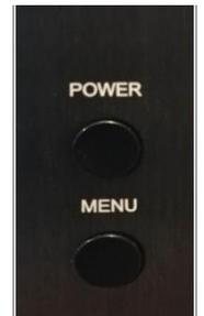
**If the screen is powered on and you still do not see anything:** ensure that the computer housed in the lower rear of the unit is switched on.
